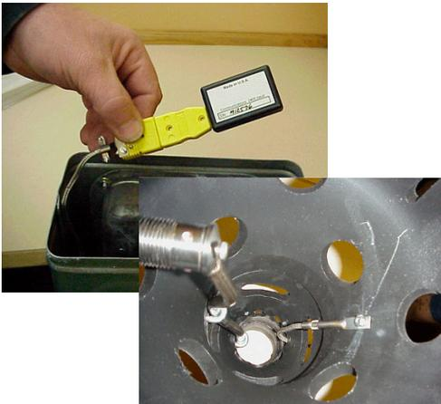
**Data Logger with Thermocouple and Flame Pilot Tube**
